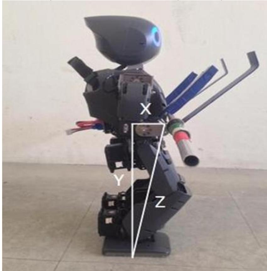
Figure 4: The robot's body is annotated with the distances used to calculate forces.
