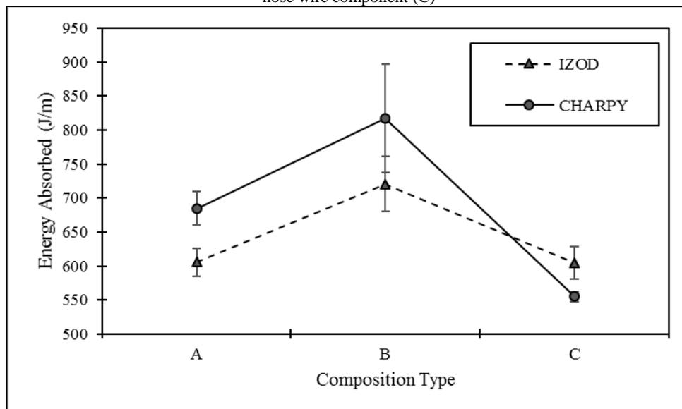
The blending of the three components in face mask waste showed different mechanical properties. In short, combination of filter and ear loop components showed better strength and toughness compared to other components. This work reported 488.43 MPa for component B tensile strength. Therefore, component B were
